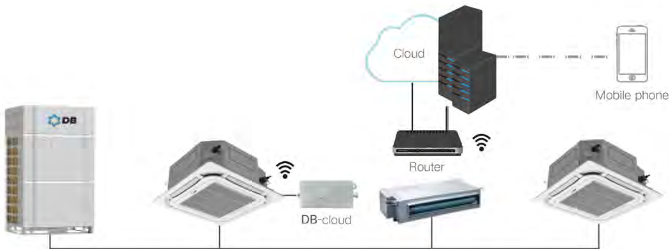
One DB-cloud can realize the control of up to 80 sets of indoor units in a system
