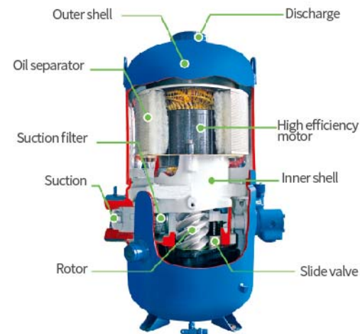
Dunham-Bush Patented Twin-screw Compressor
